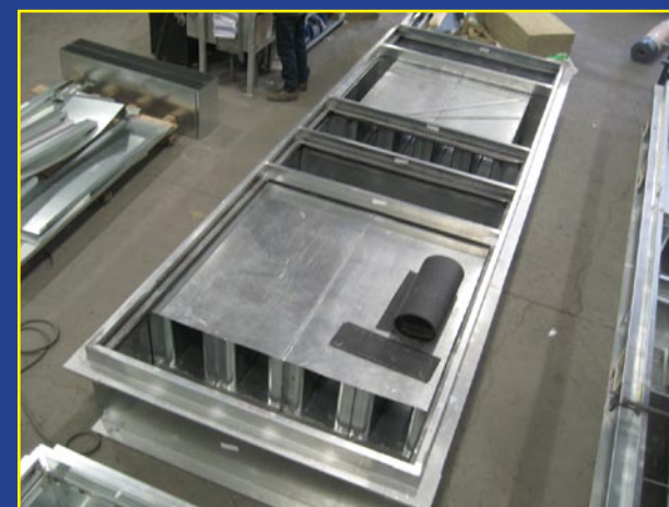
Acoustic Curb Technology for Rooftop Units
